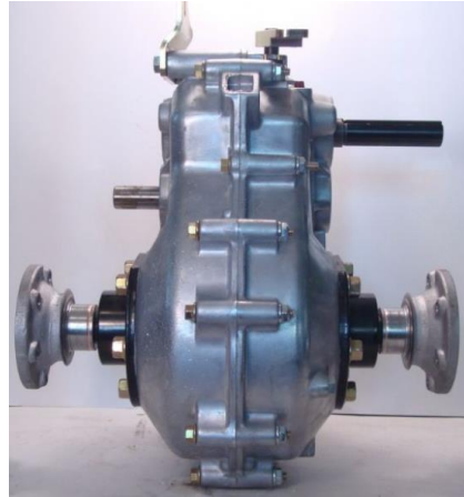
Figure 17: Dana H-12 FNR Transaxle
